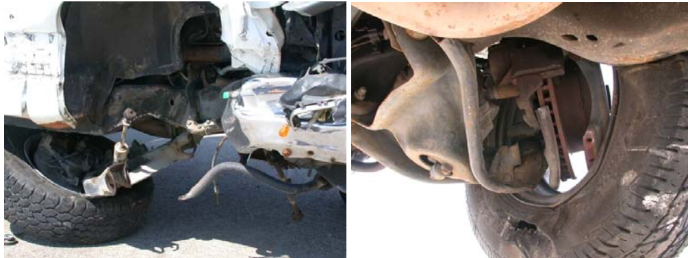
Figure 4. Lower Control Arm Deformation That Occurs During Crash Testing
