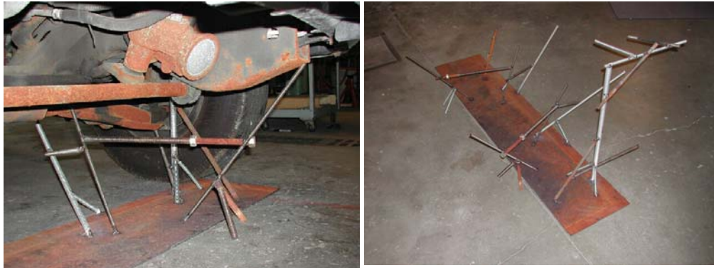
Figure 6. Structure to Find Front Suspension Mounting Points
